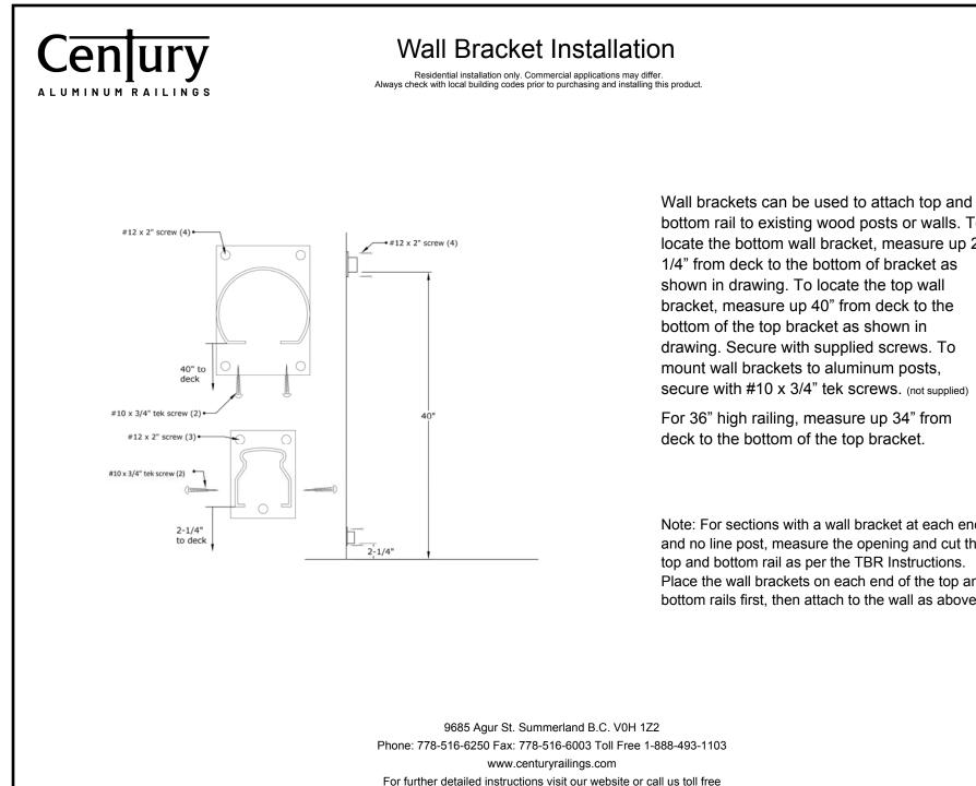
bottom rail to existing wood posts or walls. To locate the bottom wall bracket, measure up 2 1/4" from deck to the bottom of bracket as shown in drawing. To locate the top wall
