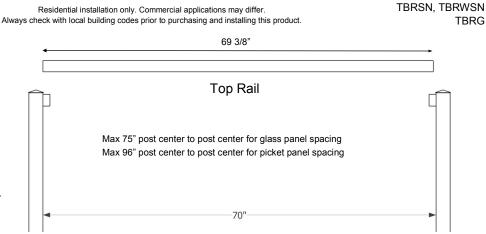
the railing at each end in line with the side of the post. Subtract 5/16" from each mark and cut both ends.
