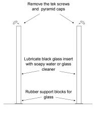
Reinstall pyramid cap and secure with the 2 #8 x 5/8" tek screws into existing holes (same for both caps)
