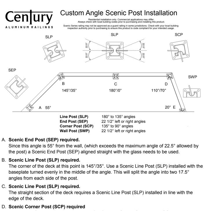
The corner of the deck at this point is  $110^{\circ}/70^{\circ}$ . Use a Scenic Corner Post (SCP) installed with the baseplate turned evenly in the middle of the angle. This will split the angle into two  $10^{\circ}$  angles from each side of the post.
