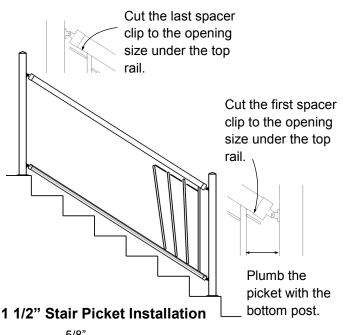
When installing 1 1/2" pickets on stairs, the corners need to be cut so the picket fits completely into the top and bottom rail channels. Failure to do so will result in the corners of the pickets protruding from the bottom and top rails.
