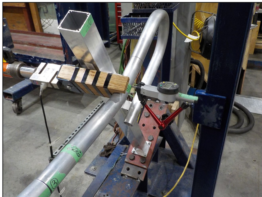
Figure 4. Horizontal – Adjacent to Post Bracket Concentrated Load
