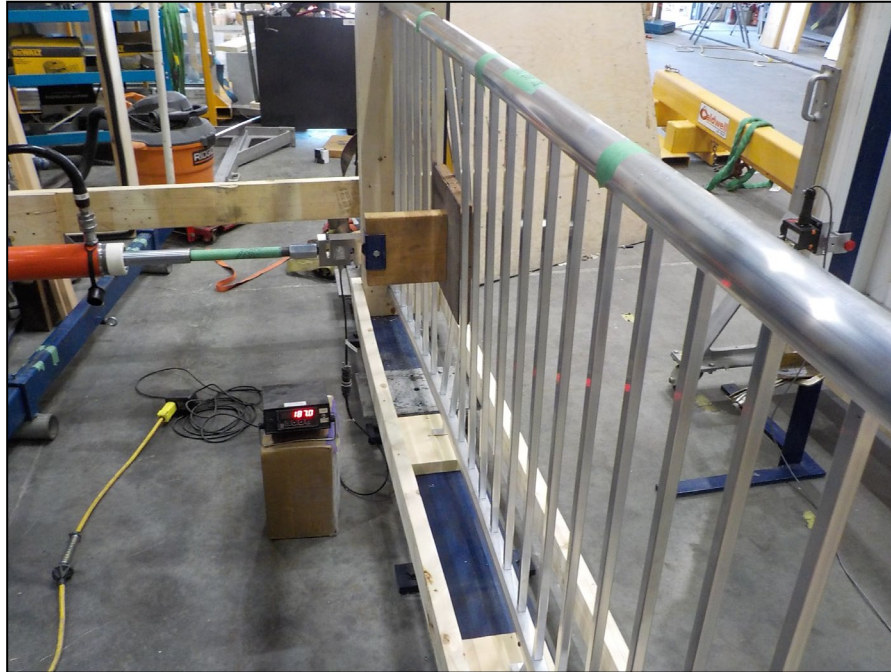
Figure 1. In-fill Load Test
