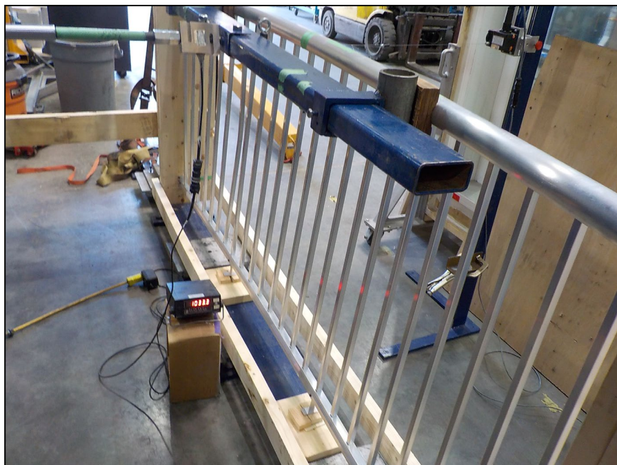
Figure 2. Horizontal Uniform Load Test
