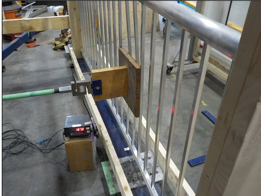
Figure 1. In-fill Load Test
