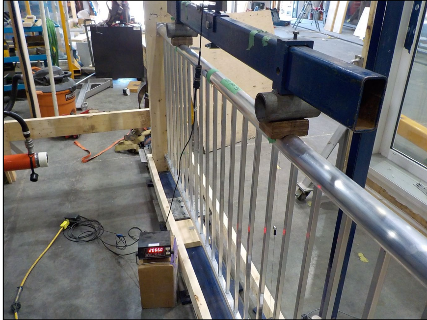
Figure 5 – 8 ft. Century Round Component Panel – Uniform Load (Vertical)
