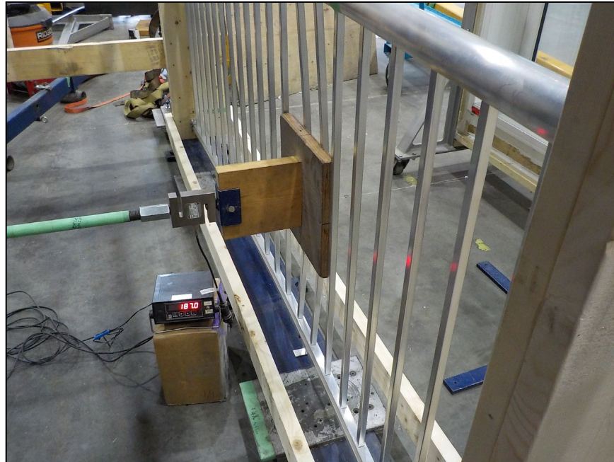
Figure 1 – 8 ft. Century Round Welded Panel – In-fill Load Test
