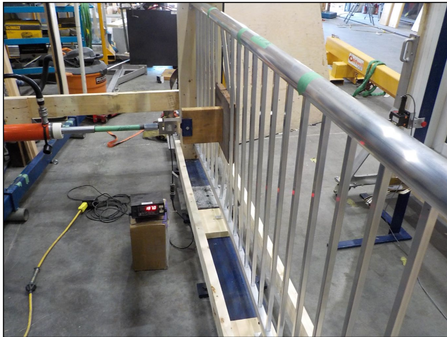
Figure 4 – 8 ft. Century Round Component Panel – In-fill Load Test
