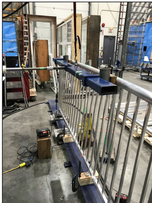
Figure 6 – Century Welded Surface: Horizontal Uniform Load Test
