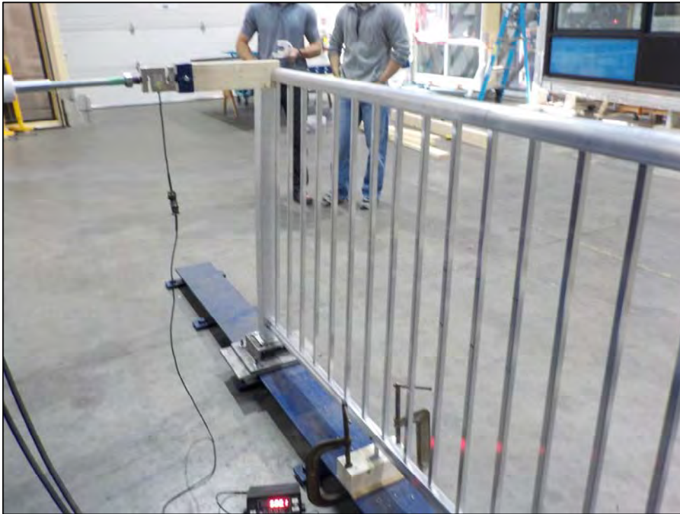
Photo 3. Adjacent to Post Connection Concentrated Load Test
