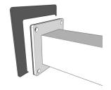
For a 5x5 baseplate, use the BPG5 6x6 gasket and trim the excess with a sharp knife
