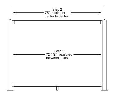
Step 3: Measure distance between inside of posts and deduct 3" from total measurement. ie: post to post measurement = 72 1/2".
