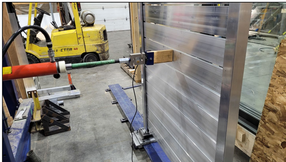
Figure 2. Privacy Wall (Deck Mount) – Horizontal – Mid-Span of Privacy Board Concentrated Load
