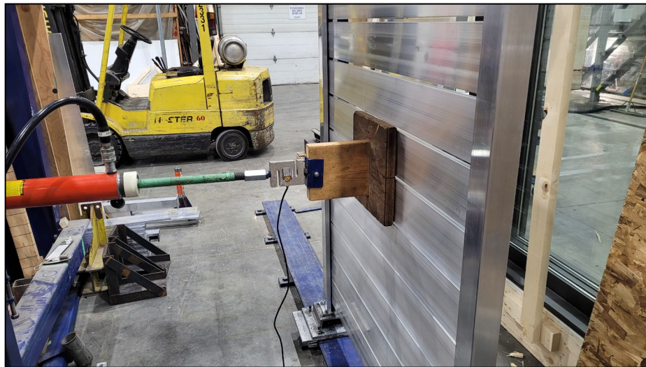
Figure 1. Privacy Wall (Deck Mount) – In-fill Load Test
