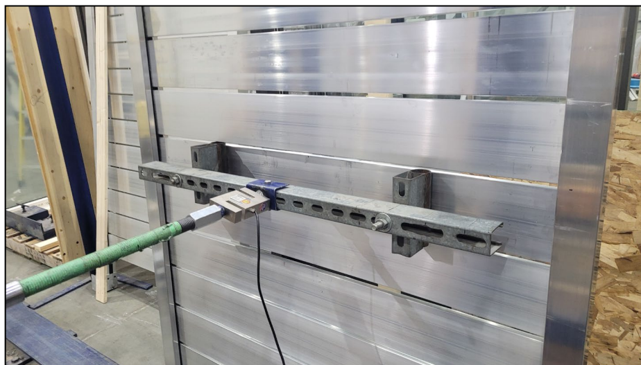
Figure 4. Privacy Wall (Deck Mount) – Uniform Load
