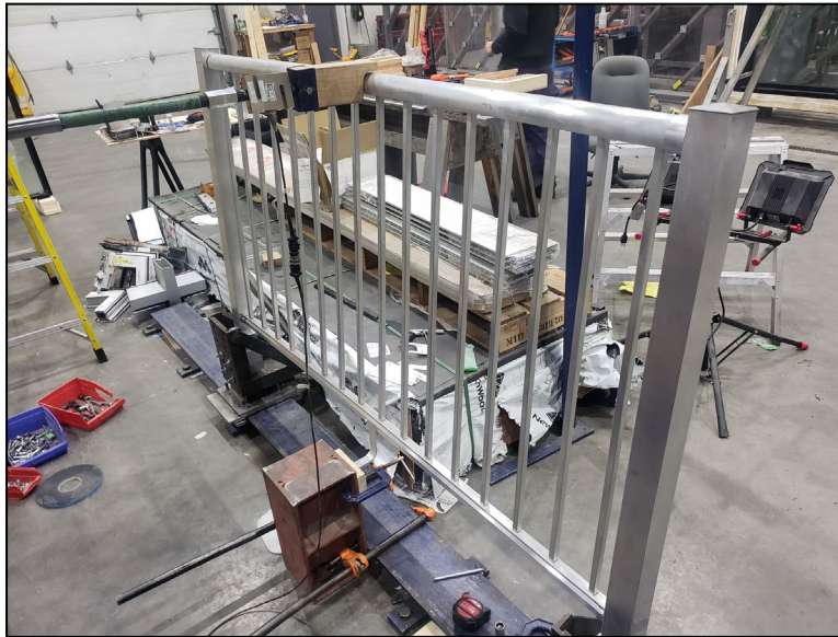
Figure 3. Horizontal –Mid-span of Top Rail Concentrated Load
