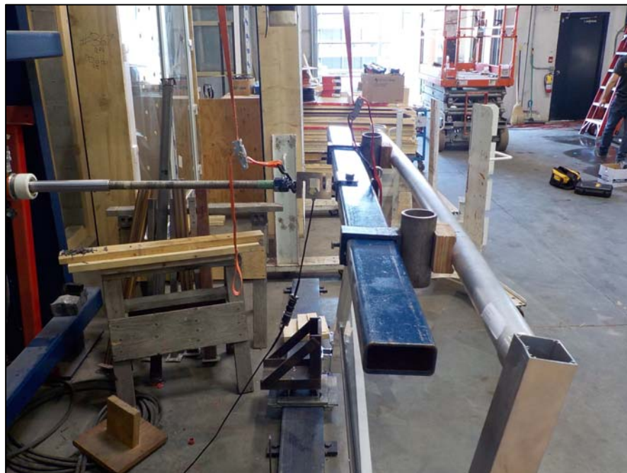
Figure 6. CTC Glass Panel – Uniform Load Test
