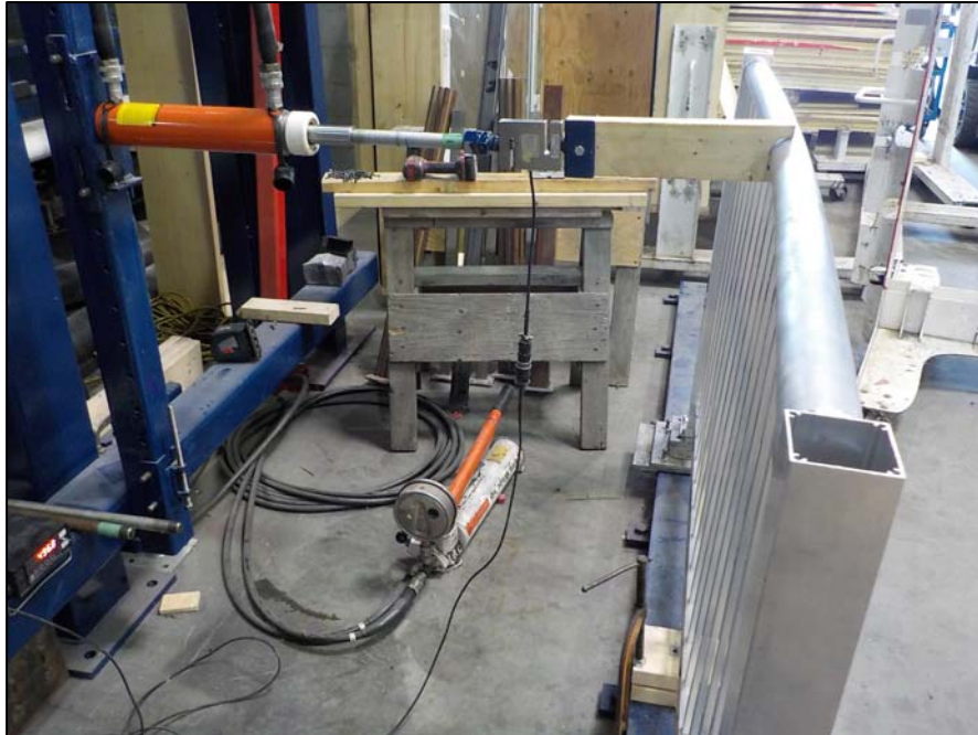
Figure 1. Century Welded Picket – Mid-Span Concentrated Load Test
