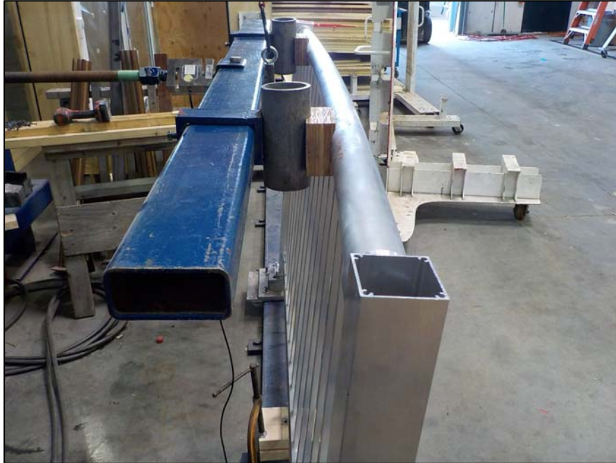
Figure 3. Century Welded Picket – Uniform Load Test
