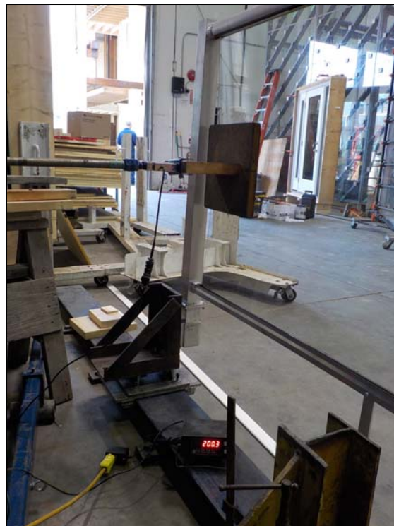
Figure 4. CTC Glass Panel – In-Fill Load Test
