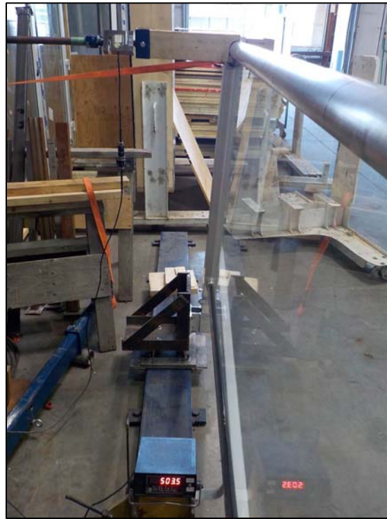
Figure 5. CTC Glass Panel – Adjacent to Post Connection Concentrated Load Test
