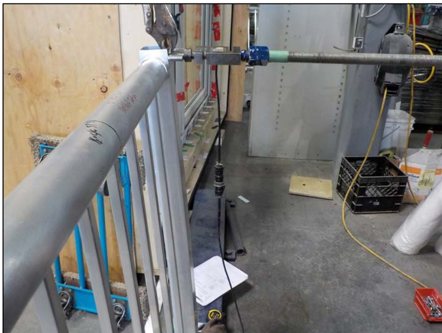
Figure 2. Century Welded Picket – Top of Post Concentrated Load Test
