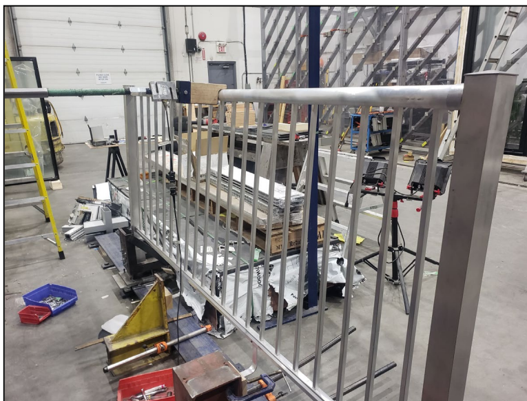
Figure 2. Horizontal – Mid-span of Top Rail Concentrated Load
