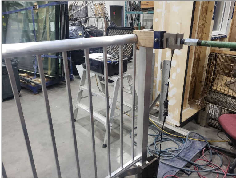
Figure 3. Horizontal – Adjacent to Post Connection Concentrated Load
