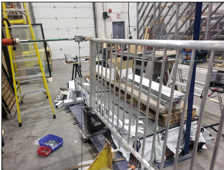
Figure 4. Horizontal – Top of Post Concentrated Load
