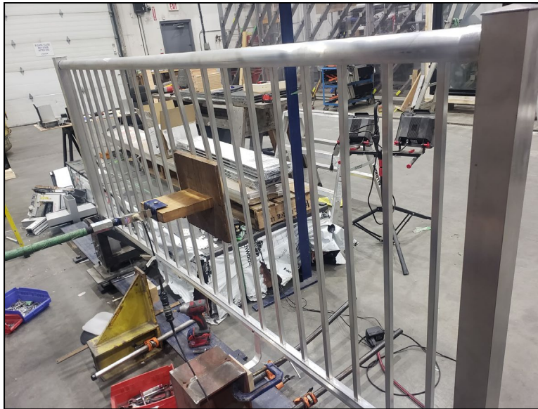
Figure 1. In-fill Load Test
