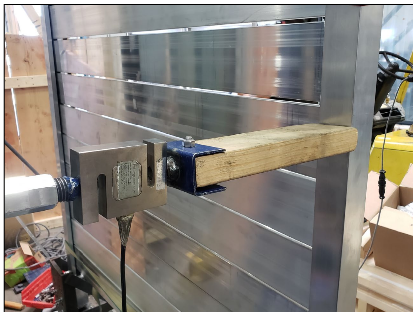
Figure 4. Post Concentrated Load
