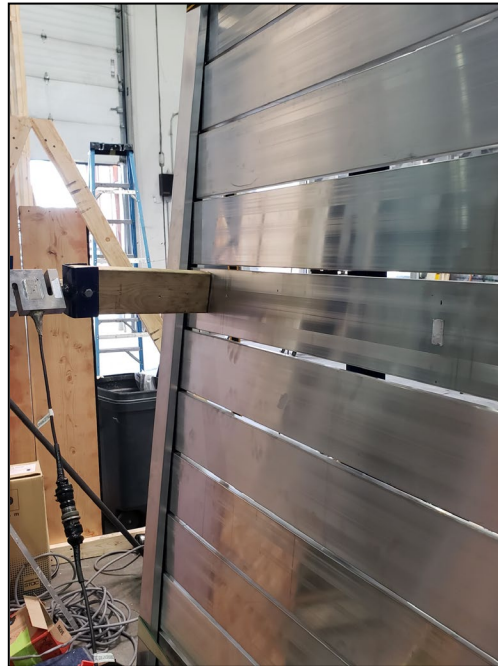
Figure 3. Adjacent to Post Concentrated Load
