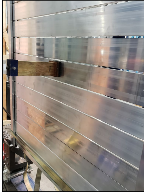
Figure 1. In-fill Load Test
