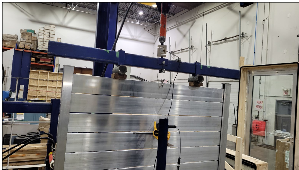
Figure 8. Privacy Wall (Fascia Mount) – Vertical Uniform Load
