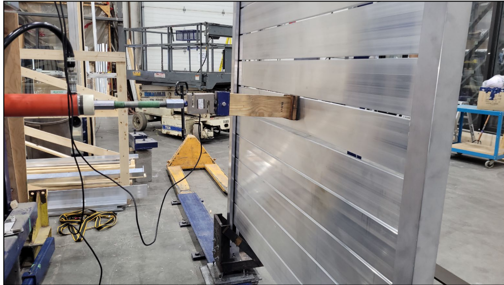
Figure 5. Privacy Wall (Fascia Mount) – In-fill Load Test
