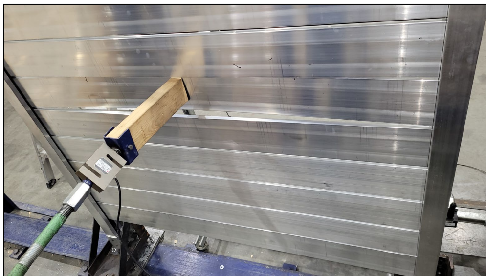
Figure 6. Privacy Wall (Fascia Mount) – Horizontal – Mid-Span of Privacy Board Concentrated Load
