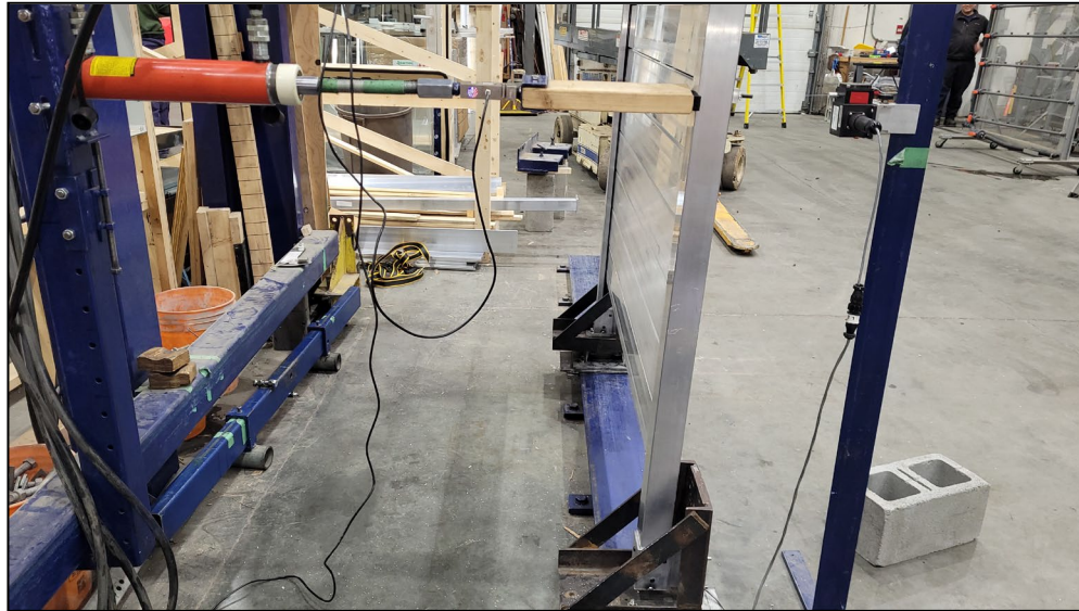
Figure 7. Privacy Wall (Fascia Mount) – Horizontal – Post Concentrated Load
