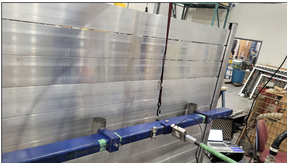
Figure 2. Privacy Wall (Deck Mount) – Horizontal Uniform Load
