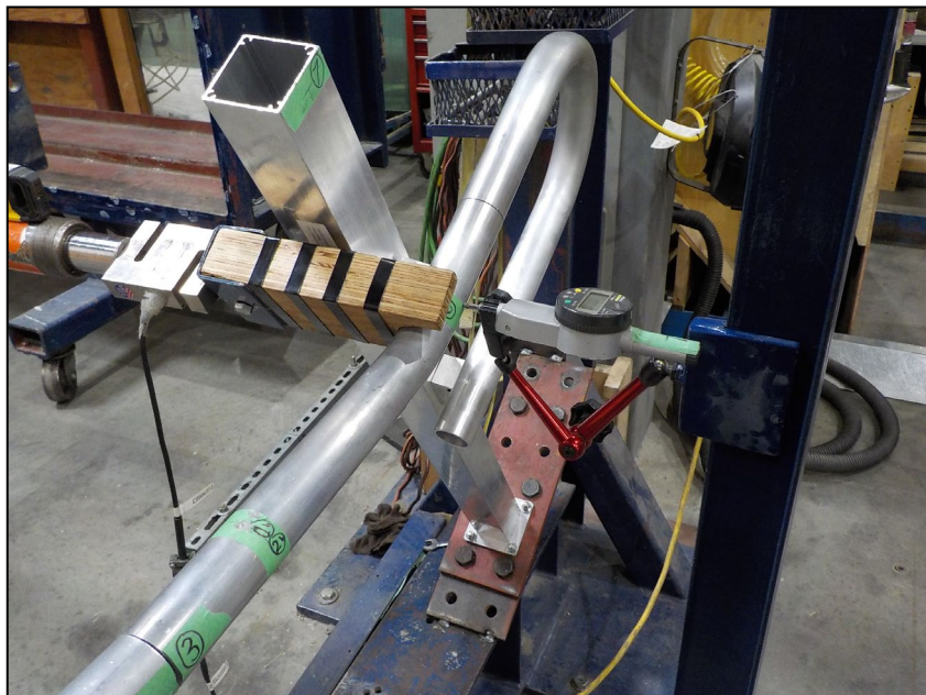
Figure 4 – Horizontal – Adjacent to Post Bracket Concentrated Load
